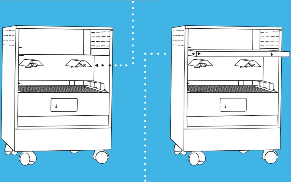
**STEP 4:** Slide in smaller **EnviroKlenz® Air Cartridge** above the UVC lights on the rails with airflow arrow facing down.
