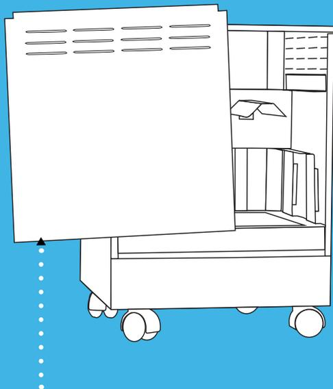
STEP 1: Make sure Air System is unplugged and slide up the back panel to insert filters.
